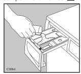
If required, pour fabric softener into the compartment marked **8** (the amount used must not exceed the "MAX" mark in the drawer). Close the drawer gently.
